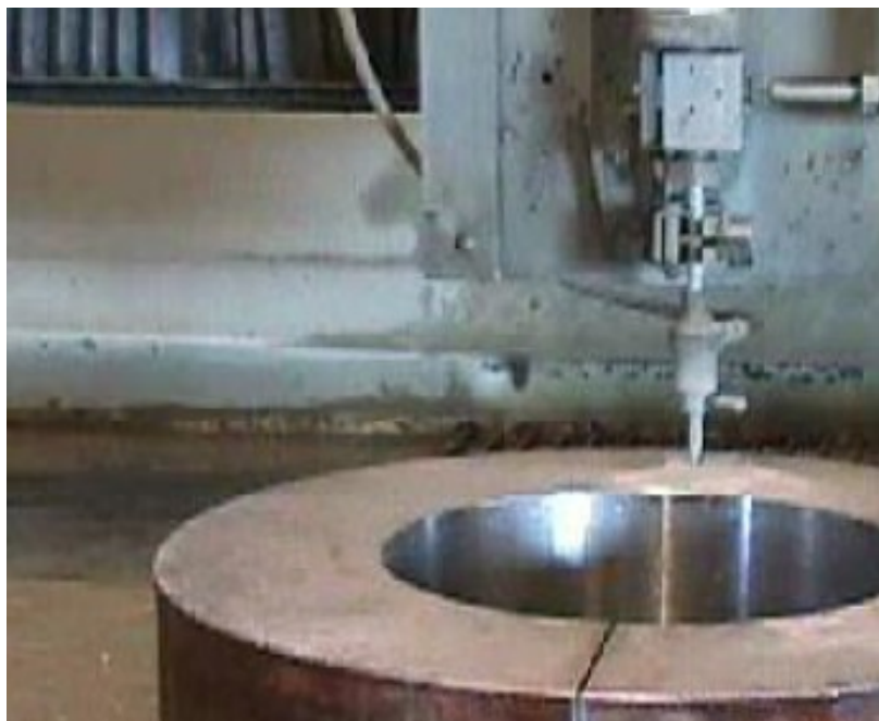
Figure 16: Abrasive water jet cutting
