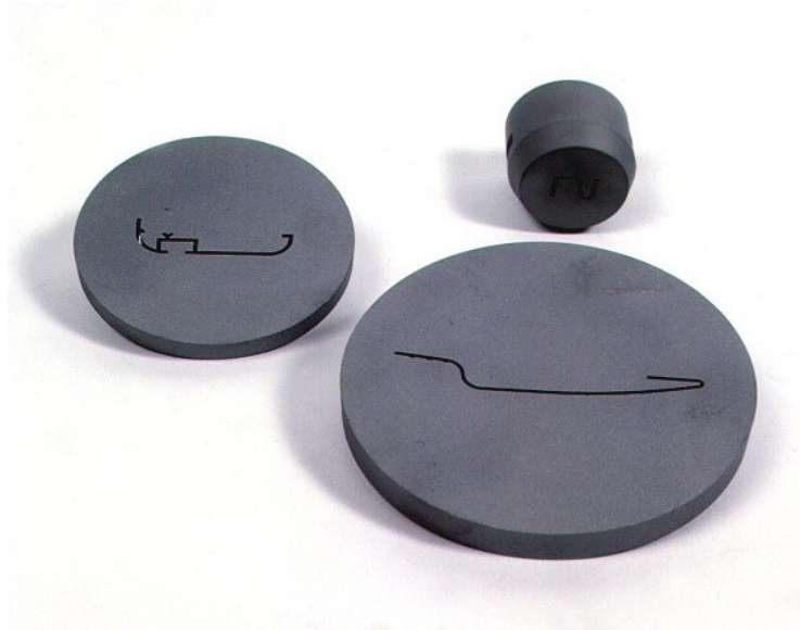
Figure 5: Sparked eroded extrusion dies
